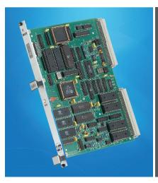
Offering reliable, highspeed operation, the Callisto IoA1 module collects analog data and performs a wide range of power system calculations.
